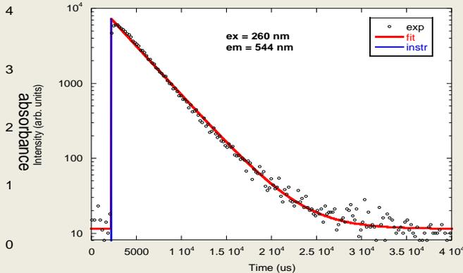
In  $Tb^{3+}$  grown crystal the emission spectrum shows full set of emission lines starting from  $^5D_3$  and  $^5D_4$  levels of  $Tb^{3+}$ . PLE spectrum shows 4f-5d transition of  $Tb^{3+}$  below 280 nm, fingerprint of  $Gd^{3+}$  absorption lines at 305-210 nm, the broad band around 450 nm might be due to  $Ce^{3+}$  contamination. Decay time of 544 nm line is 3.3 ms, consistent with strongly forbidden character of  $Tb^{3+}$  4f-4f transitions
