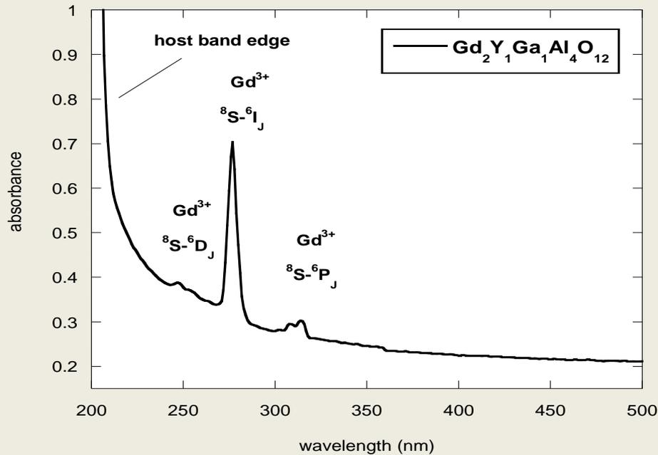
Absorption spectrum of **Gd<sub>2</sub>Y<sub>1</sub>Ga<sub>1</sub>Al<sub>4</sub>O<sub>12</sub>**. Intense Gd<sup>3+</sup>-related peak at 270 nm as well as host lattice absorption region ( $\lambda \leq 220$  nm) are evident.
