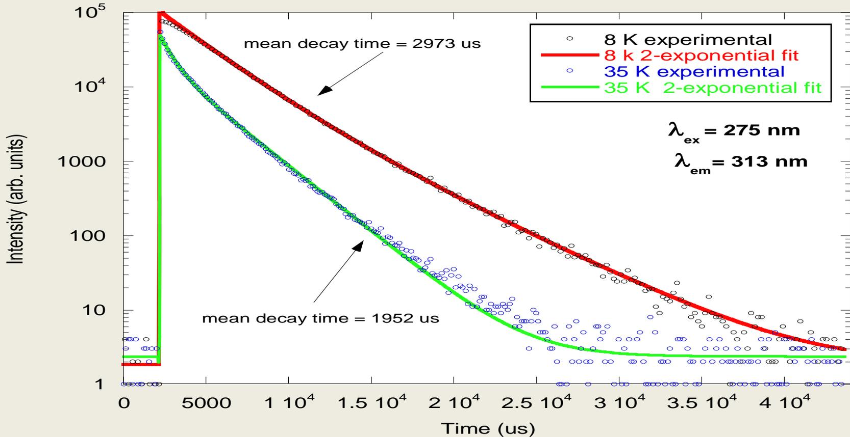
Decay curves of the intrinsic  $\text{Gd}^{3+}$  emission of  $\text{Gd}_2\text{Y}_1\text{Ga}_1\text{Al}_4\text{O}_{12}$  single crystals as a function of temperature.
