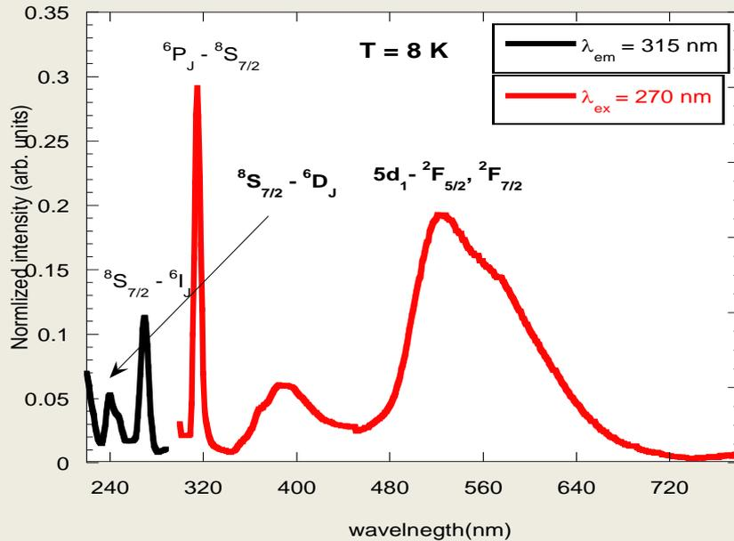
PLE spectrum monitored at maximum of  $\text{Ce}^{3+}$  emission. Presence of weak line at 270 nm ( $\text{Gd}^{3+}$  – related) confirm the energy transfer from  $\text{Gd}^{3+}$  to  $\text{Ce}^{3+}$
