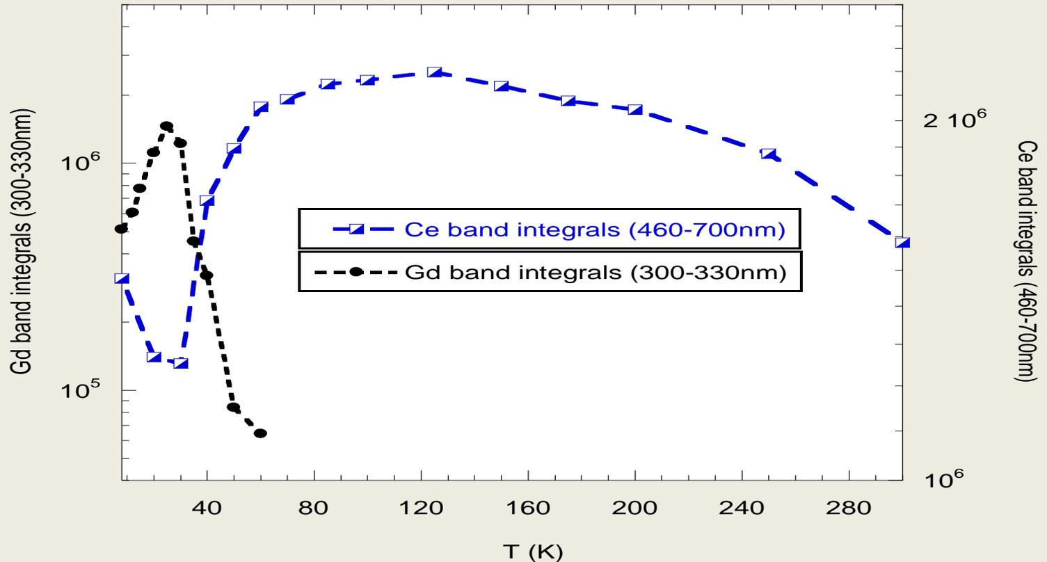
Gd and Ce – related emission bands in **Gd<sub>3</sub>Ga<sub>3</sub>Al<sub>2</sub>O<sub>12</sub>:Ce** upon excitation at  $^8S \rightarrow ^6I_J$  absorption band of Gd<sup>3+</sup> as a function of temperature
