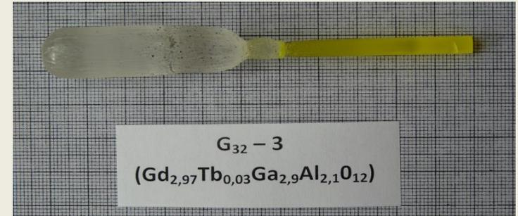
Crystals grown by Czochralski method in **IP Prague laboratory** (seeds from C&A Japan)
